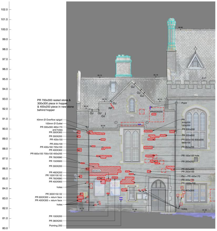
**Tabric Repair to South West Elevation**Scale 1:100
